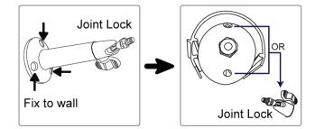
Step3: Fasten the camera with the joint lock to the bracket.
